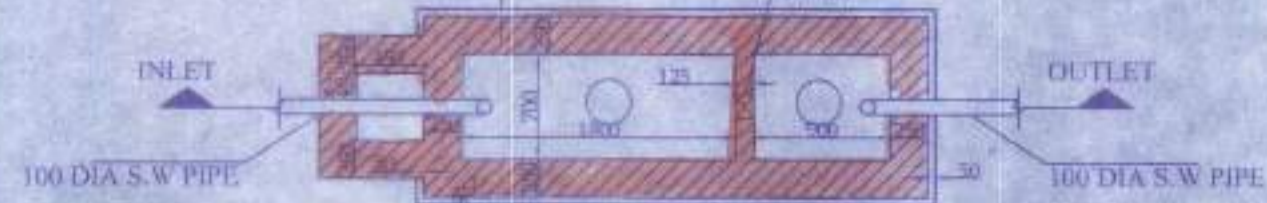
PLAN OF SEPTIC TANK (for 20 users) SCALE - 1:50
